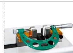
zero setting and calibration of micrometers
